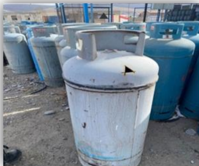
Fig. 10. Gas cylinder top dome damage
