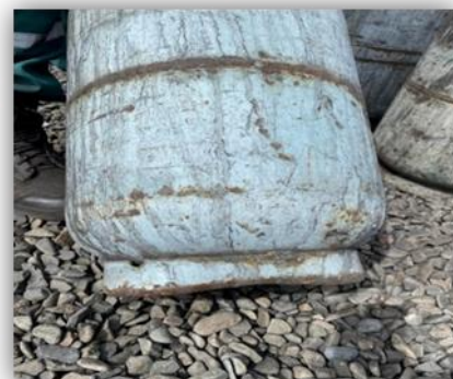
Fig. 13. Gas cylinder base ring damage
