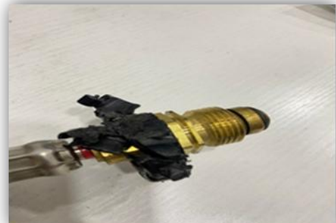
Fig. 11. Gas cylinder valve damage
