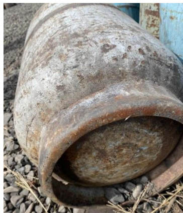
Fig. 8. Corrosion of the gas cylinder base ring.
