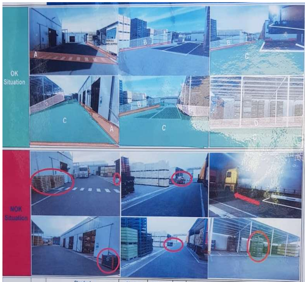
Fig. 5 The application of 5S in the external storage area
