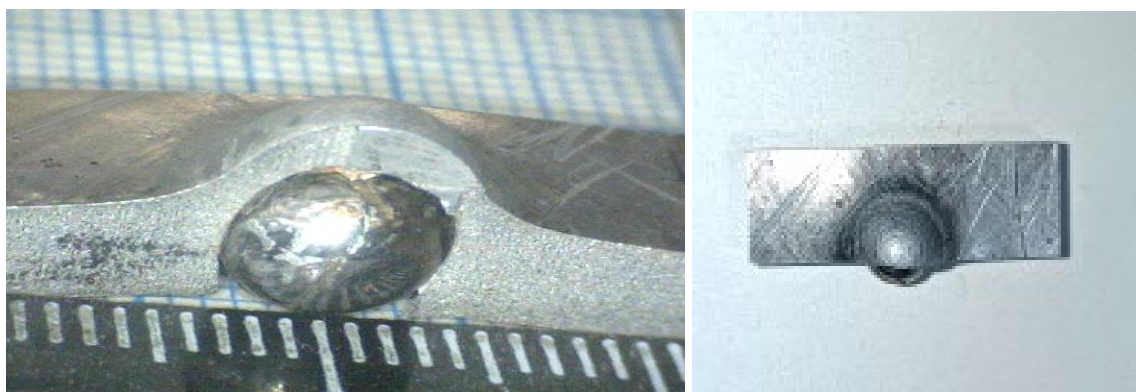
Figure 1. Steel ball stuck in a duralumin plate: (a) View from the side section; (b) View from the side of a possible departure.
