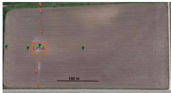
Fig. 4. Google Earth satellite image of the D#2 well and measurement points of H 2 concentration in soil (Kansas, USA) [5].
